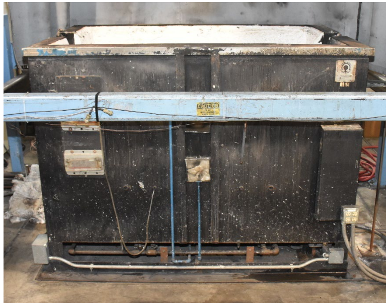
Figure 2.1. FPL Intermediate-scale horizontal furnace without lid or specimen installed.
